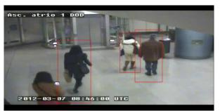
**Static-luggage detection**. The algorithm relies on a multi-layer background subtraction method by distinguishing recent background layers from old and long term background layers and foreground regions. It is enhanced by a human detection algorithm to remove false alarms due to people waiting and hence remaining static for quite some time.
