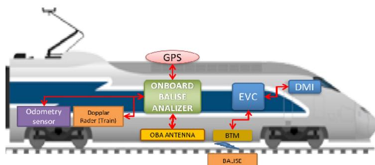
Fig 1- Schematic placement of the OBA on the train. There is no BTM interference
