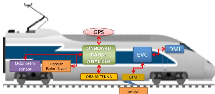
Fig 1- Schematic placement of the OBA on the train. There is no BTM interference
